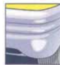
Bumper with excessive scuffing.
