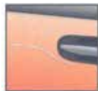
Isolated scratches over 50mm in length which penetrate to metal or primer.
